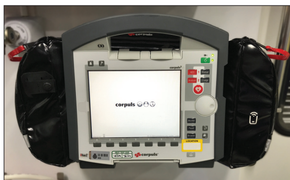
Figure 22.6 A Corpuls3 monitor/defibrillator commonly used by ambulance services.
