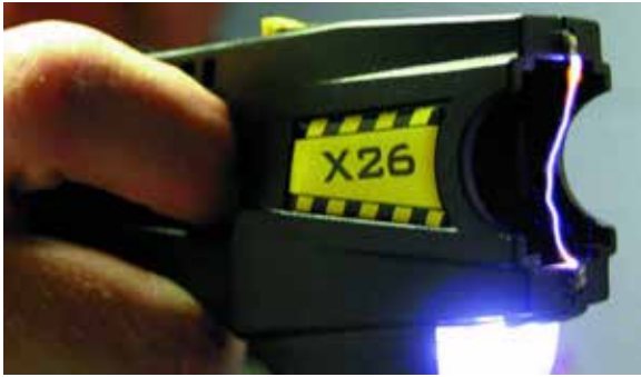
Figure 6.5 A Taser being ‘arced’. Note that there is no cartridge installed on the device. Source: jasonesbain (Taser) [CC BY 2.0], via Wikimedia Commons.
